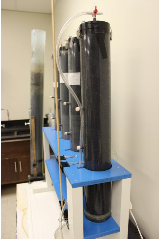
Photo caption: Pictured above are column tests performed in the lab of Valentine Nzengung. He and his graduate student are exploring the use of other wastes (aluminum cans, biochar, and slags) to stabilize deposits of coal ash from power plants.
