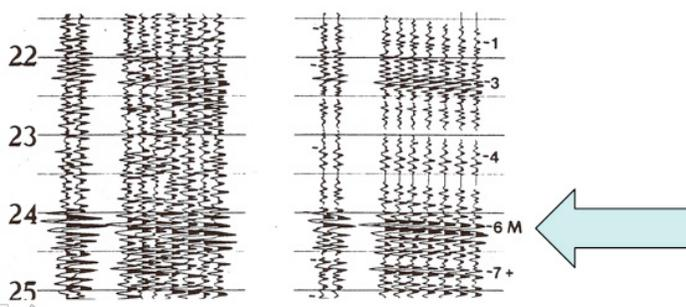
*Wide-angle reflections generated by a quarry blast in the central Appalachians, recorded with a short-aperture array (duration: 0.25 seconds; distance: about 124 km). Before (left) and after (right) coherency filtering. Migration of event "M" (interpreted as the Moho) suggests a crustal thickness of 44 km beneath the Conestoga Valley of southeastern Pennsylvania (*Hawman & Phinney, 1992b*).*
